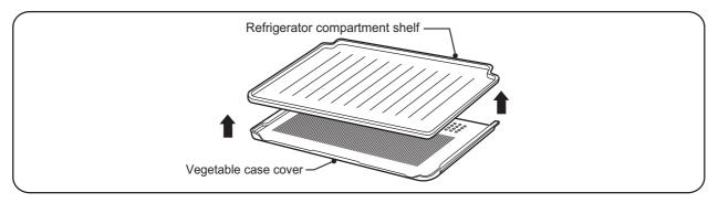
Insert the attached Vegetable case cover and compartment shelf into the rails (both left and right) upon the vagetable case. Then insert the vegetable case.
