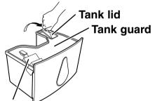
Floating element Do not remove or dismantle the float.
