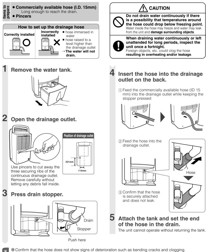
Confirm that the hose does not show signs of deterioration such as bending cracks and clogging
