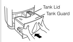
Check that the lid and guard are secure. Slide the tank in with both hands.
