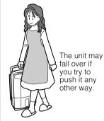
Always move the unit by rolling it on its castors. Before moving the unit, first make sure to remove water from the drainage tank and close the louvre.
